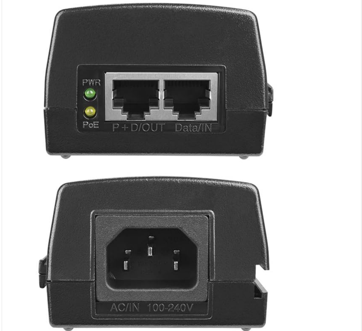
Figure 4: Front and Back Panels. This image displays the injector's front panel with the PWR and PoE indicator LEDs, along with the Data/IN and P+D/OUT Ethernet ports. The back panel shows the AC power input.
