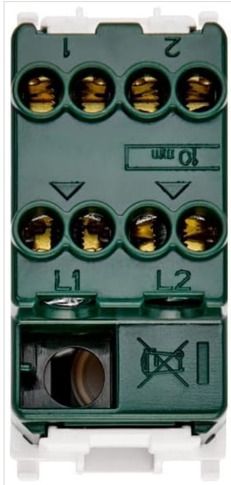
Figure 1: Back view of the Vimar 14015 switch with wiring terminals. Terminals L1 and L2 are for incoming power lines, and terminals 1 and 2 are for outgoing load connections in a 2-way circuit.
