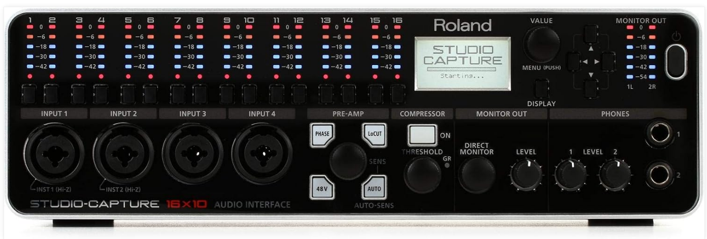
Figure 1: Front Panel of the Roland STUDIO-CAPTURE UA-1610. This image displays the front panel of the Roland STUDIO-CAPTURE UA-1610 audio interface, highlighting its 16 input channels, pre-amp controls, monitor output section, and dual headphone outputs. The central display shows 'STUDIO-CAPTURE Starting...' indicating power-up.
