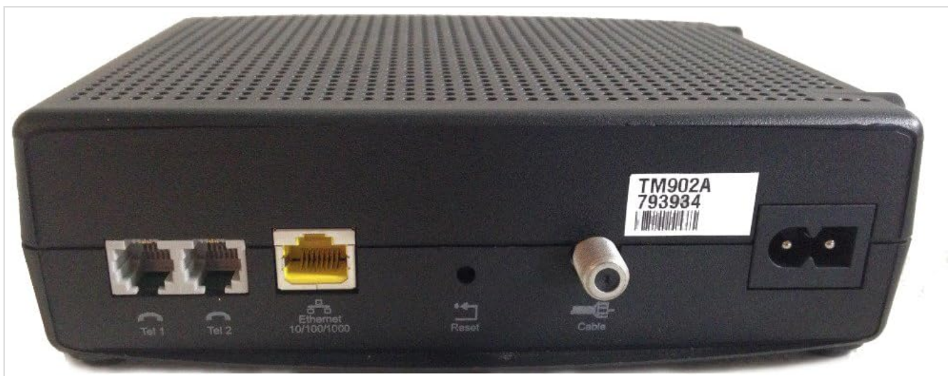
Image: Rear view of the ARRIS TM902A Telephony Modem, showing the Tel 1, Tel 2, Ethernet, Reset, Cable, and Power ports. A label with "TM902A 793934" is visible.
