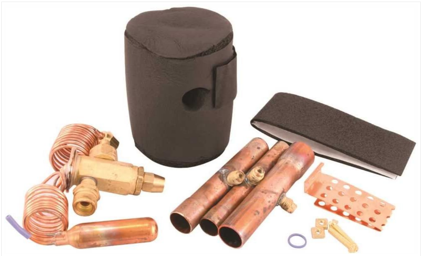
Figure 1: Goodman TXV kit. This image displays the main thermal expansion valve body, the coiled copper sensing bulb with its capillary tube, the external equalizer line, and a black insulating sleeve designed to cover the sensing bulb. Also visible are various copper pipe sections and fittings, indicating the components required for a complete installation.
