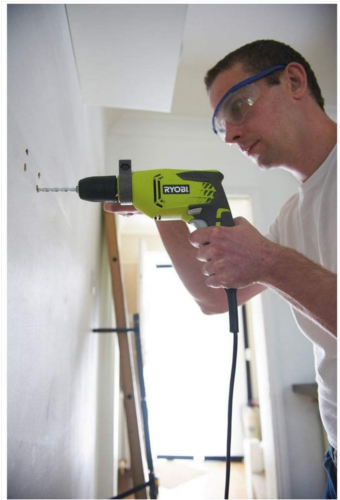
Image 3.2: Side view of the Ryobi RPD500-G, showing the main handle with trigger and mode selector.
