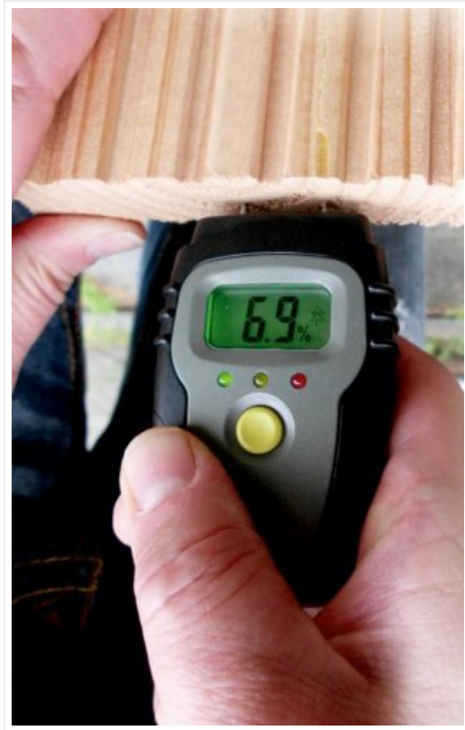
Figure 4: A close-up view of the Werkzeyt B29820 moisture meter with its probes inserted into a piece of wood, displaying a reading of "6.9%".
