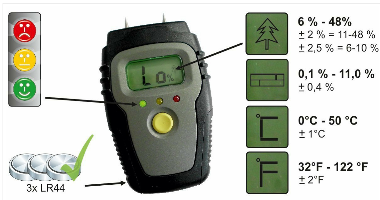
Figure 2: This image illustrates the device's display showing "Lo %" and the indicator lights. It also details the measurement ranges for wood (6%-48%), building materials (0.1%-11.0%), and temperature in Celsius (0°C-50°C) and Fahrenheit (32°F-122°F). The bottom left confirms the use of 3x LR44 batteries.
