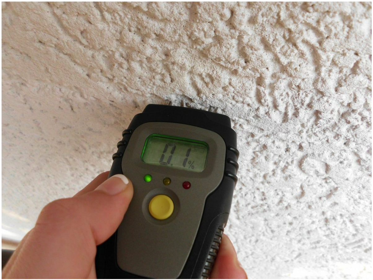
Figure 6: The Werkzeyt B29820 moisture meter with its probes inserted into a textured wall or building material, displaying a reading of "0.1%".
