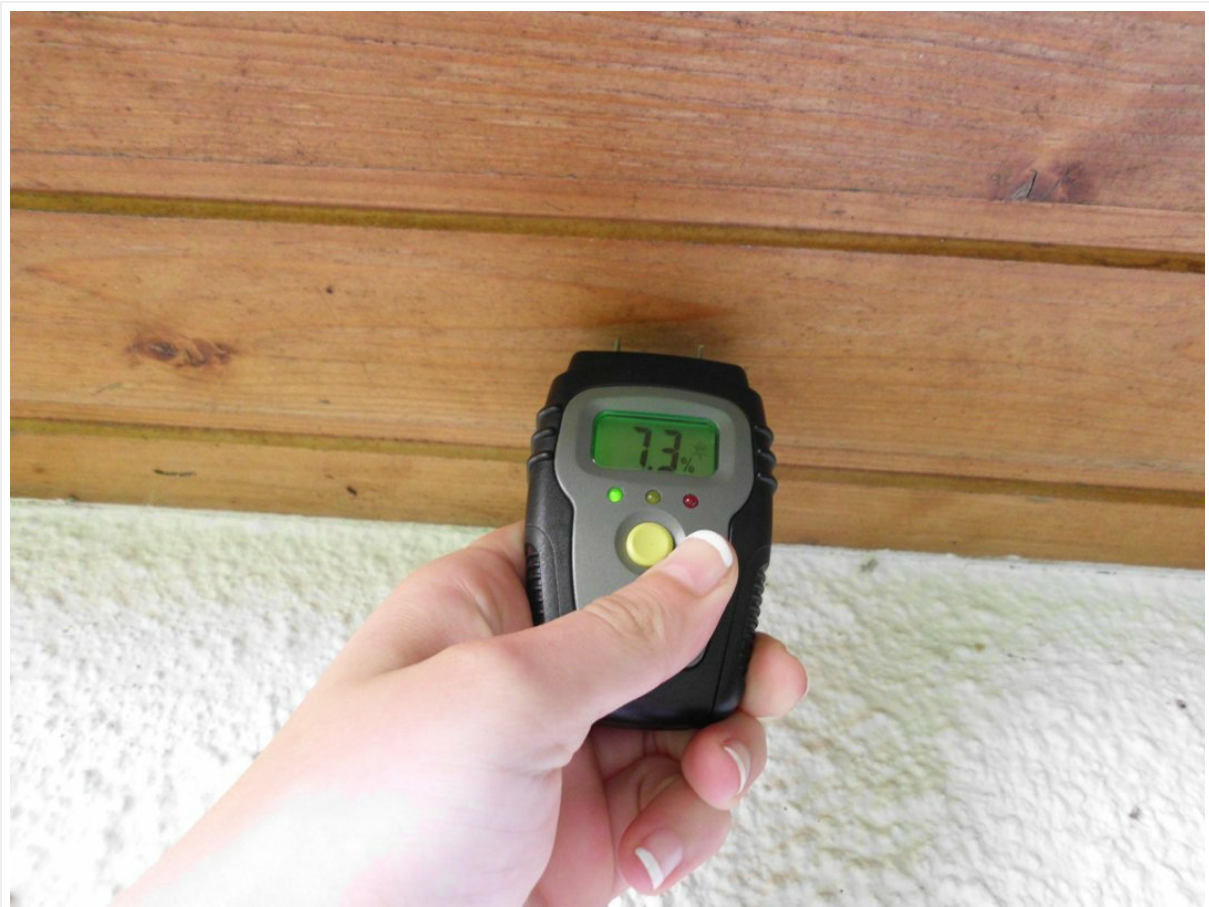
Figure 5: The Werkzeyt B29820 moisture meter being used to measure the moisture content of a wooden panel, showing a reading of "7.3%".
