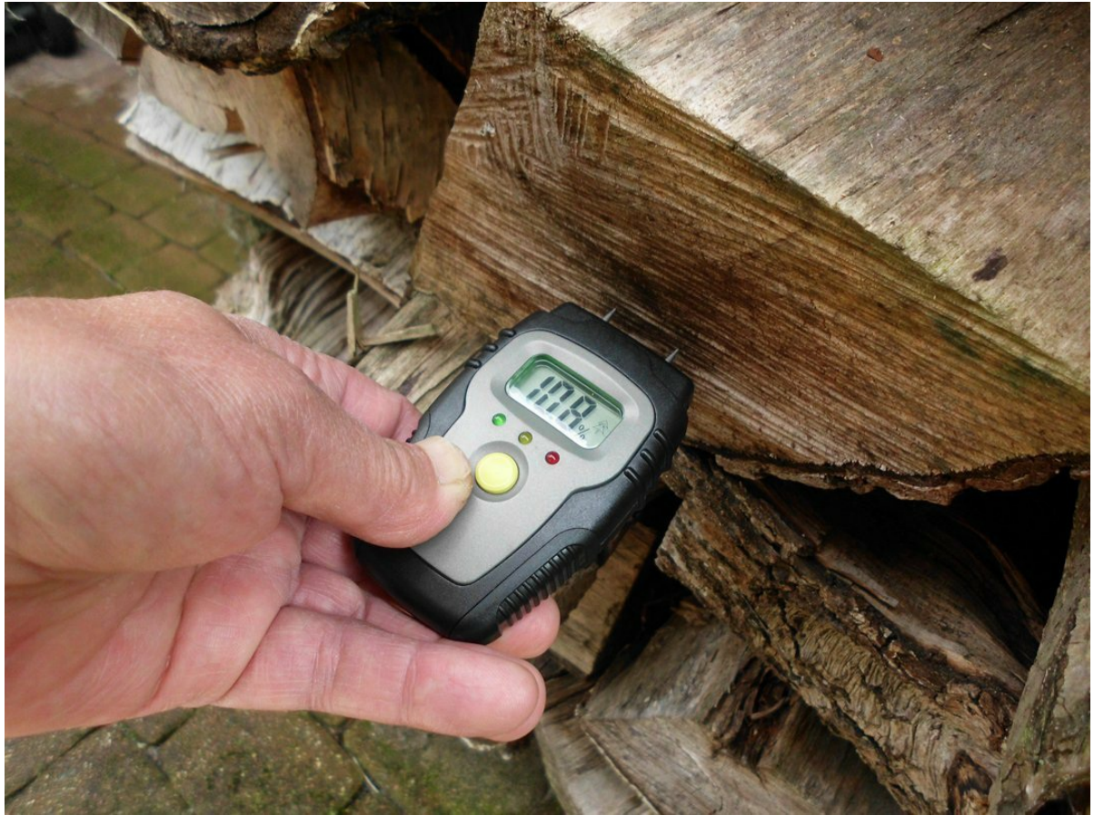
Figure 3: A hand holding the Werkzeyt B29820 moisture meter, pressing its probes into a piece of firewood to measure its moisture content. The display shows "10.8%".
