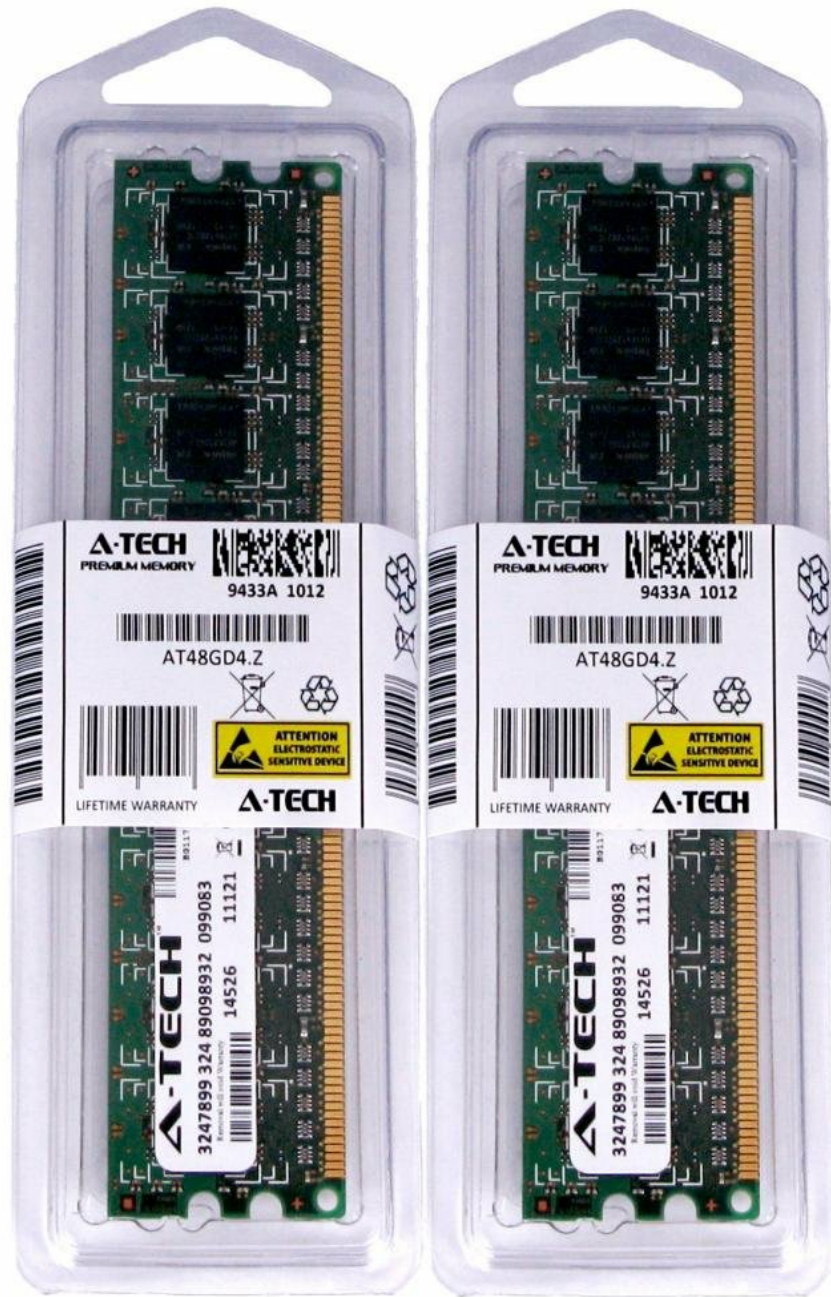
Image: Two A-Tech DDR2-667 RAM modules, part of the 4GB upgrade kit.
