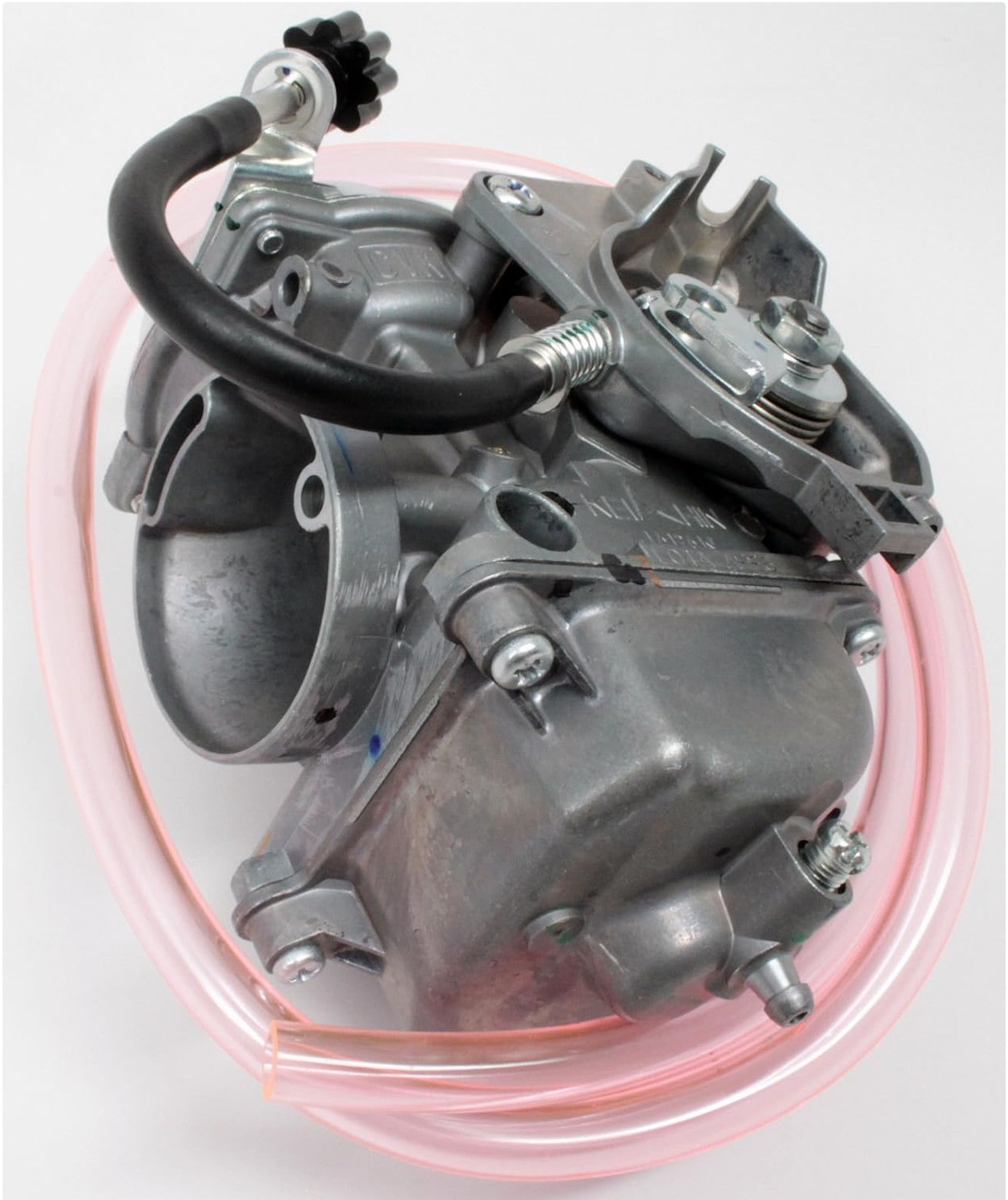
Figure 3.1: Side view of the Keihin CVK 32 Carburetor (0470-448) showing the main body, throttle linkage, and clear fuel overflow line.
