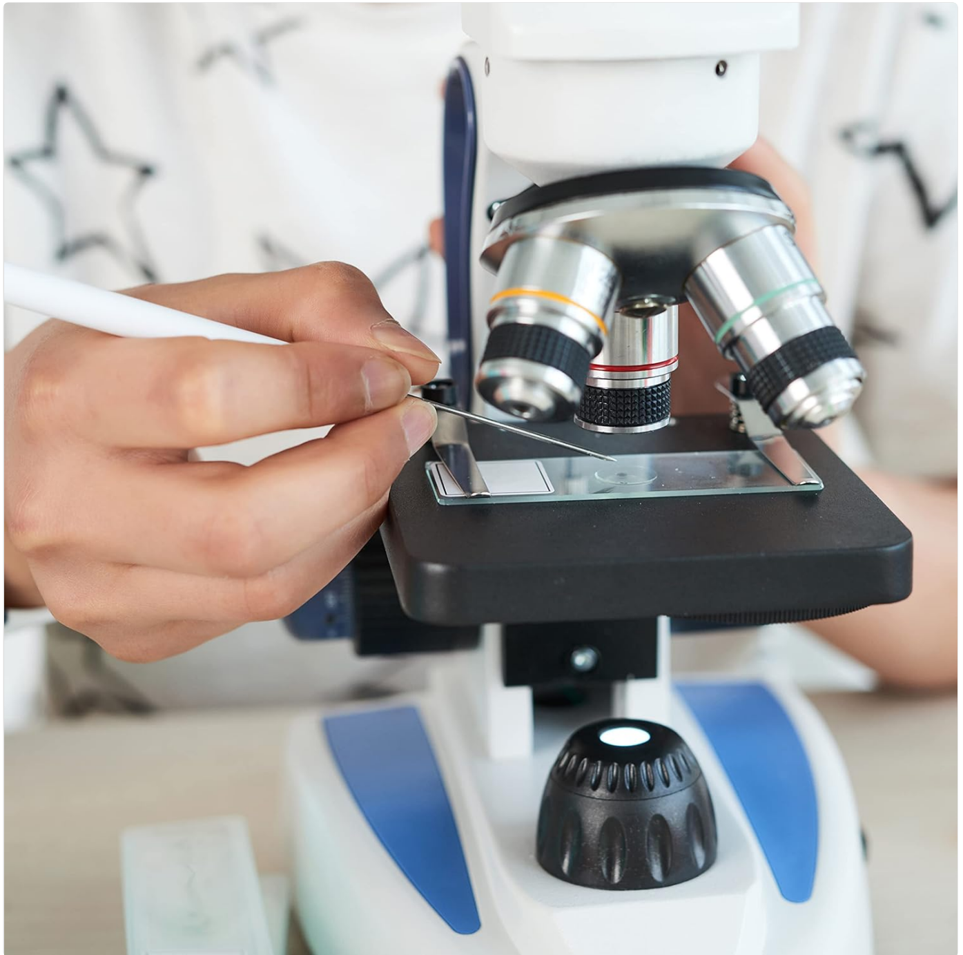
Figure 2: User placing a specimen slide on the microscope stage. This image illustrates the proper method for securing a slide using the stage clips on the plain stage.
