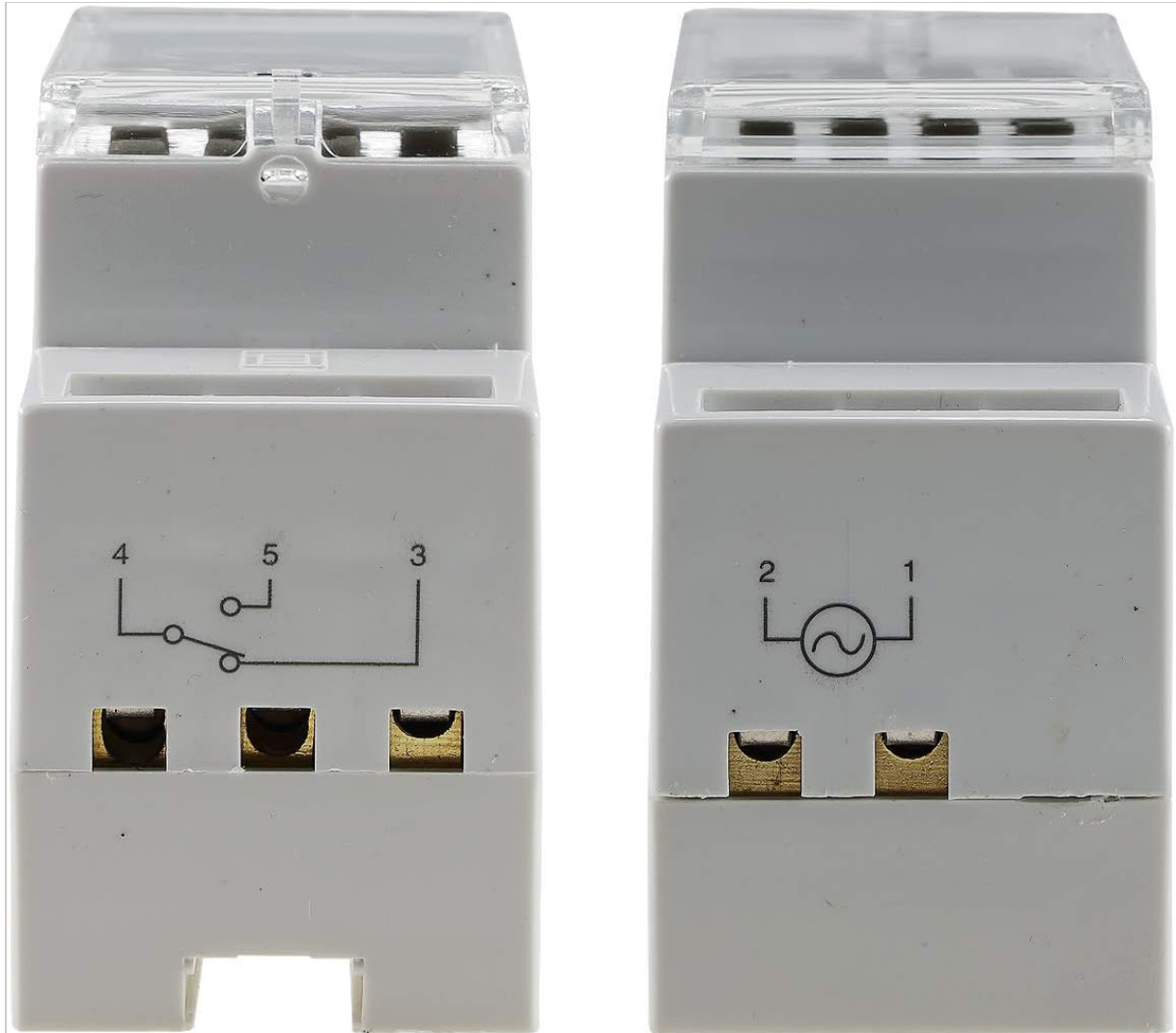
Figure 3: Detailed view of the wiring terminals on the ChiliTec Digital DIN Rail Timer, showing connections for power input (1, 2) and switch contacts (3, 4, 5).
