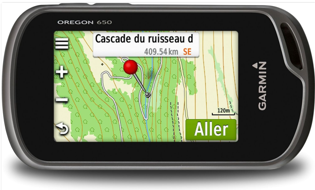
Figure 4.1: Map display on the Oregon 650, showing a marked location and navigation option.
