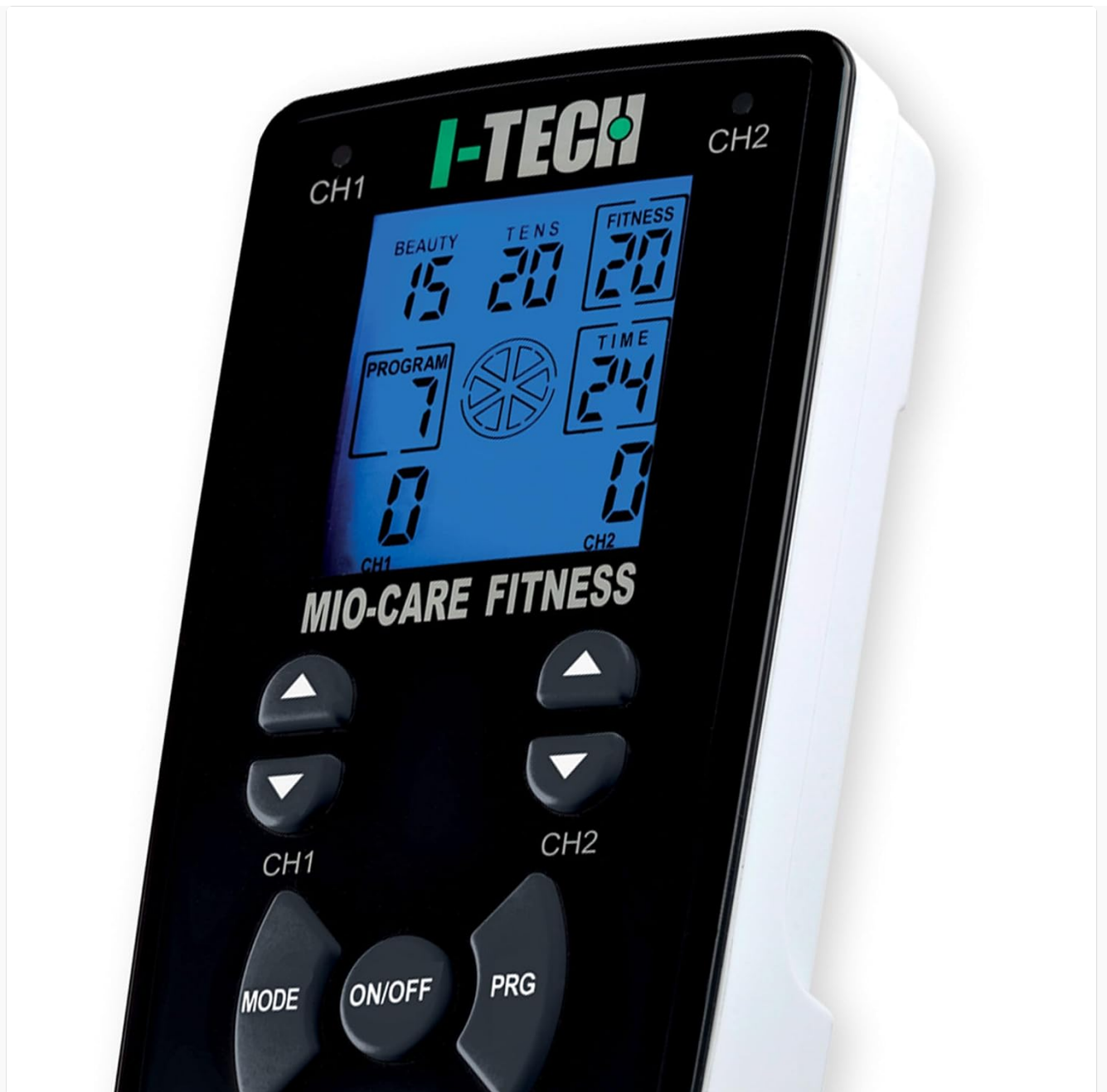
Image: A detailed close-up of the electrostimulator's screen, highlighting the program selection, time remaining, and intensity controls for both channels (CH1 and CH2).
