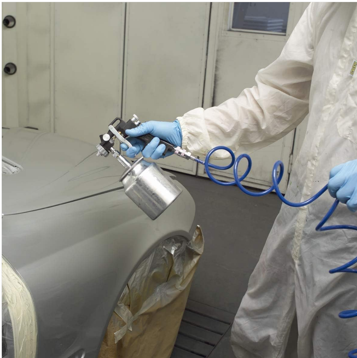
Figure 3: Example of the FERM ATM1040 Paint Spray Gun in use, demonstrating proper technique on a vehicle panel.
