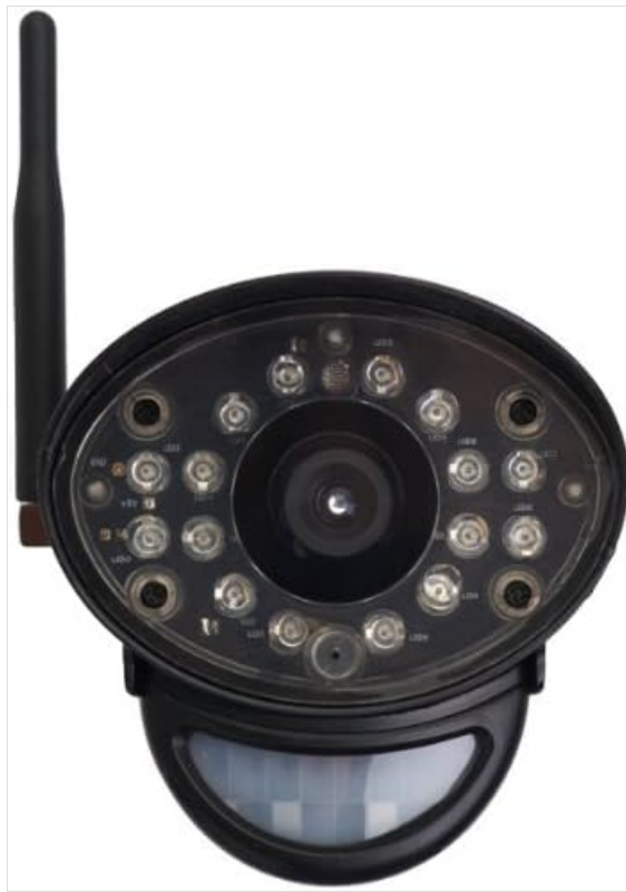
Figure 3.2: Close-up front view of the camera, highlighting the lens, infrared LEDs, and the motion sensor below.
