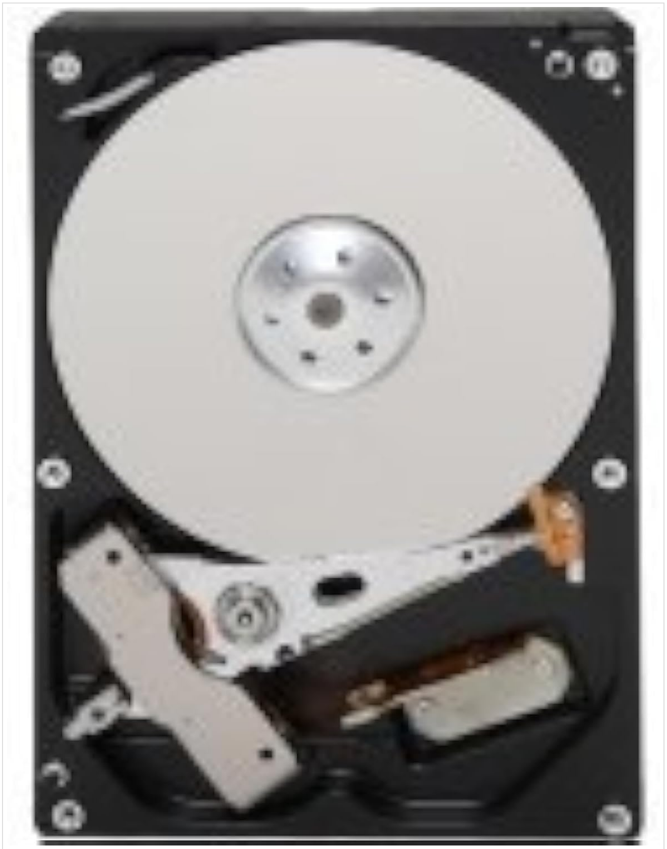
This image displays the internal components of the Toshiba DT01ACA100 hard drive, including the circular data platter and the read/write head mechanism. This view is for illustrative purposes only; the drive should not be opened by the user.
