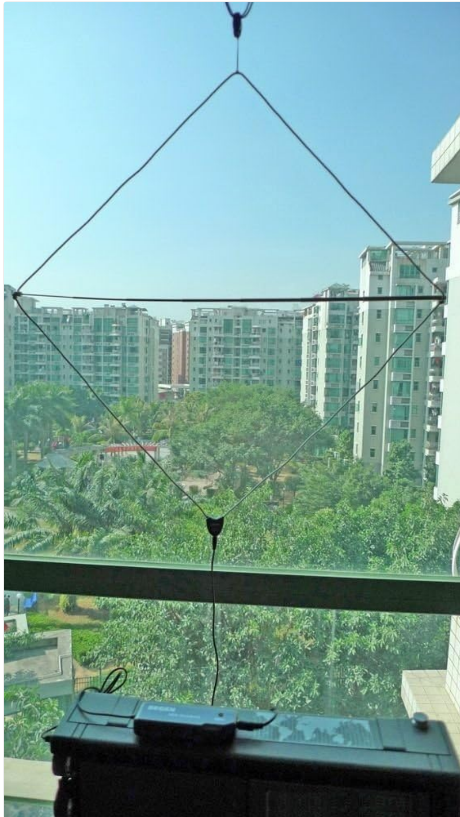
Image: Example of the DEGEN DE31MS antenna loop mounted on a window for optimal signal reception.
