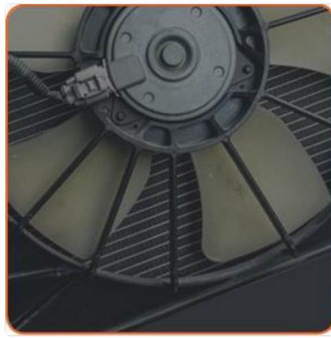
Images: Illustrative diagram showing the typical placement of a radiator fan assembly within a vehicle's engine bay, and a close-up view of the fan blades and radiator fins.
