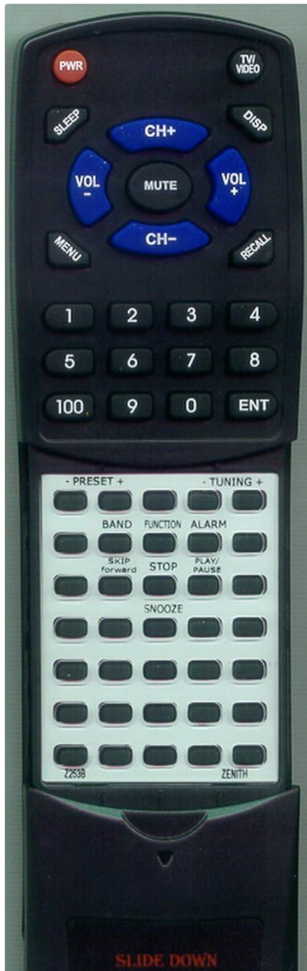
Image: Front view of the Redi-Remote replacement remote control. The top section features primary controls like Power, Volume, Channel, and Number Pad. The bottom section, initially covered, slides down to reveal additional function buttons.
