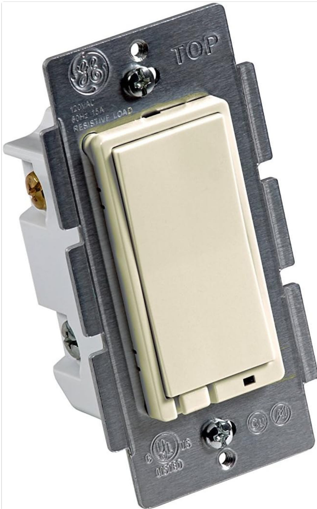
Figure 1: Front view of the GE Z-Wave On/Off Relay Switch (Model 45609) without a wallplate, showing the rocker switch and mounting bracket. The "TOP" indicator is visible at the top of the metal bracket. Electrical ratings (120VAC, 60Hz, 15A Resistive Load) are printed on the side.
