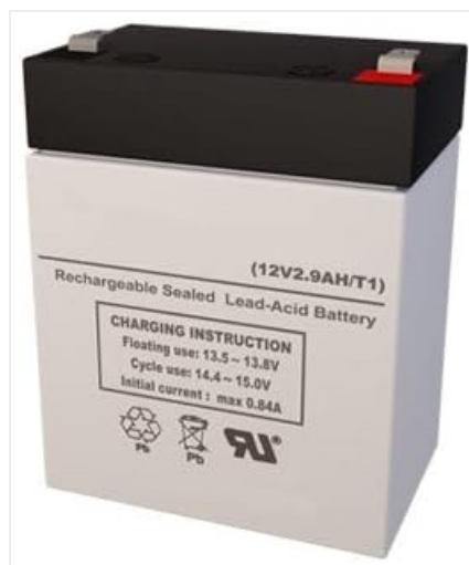
Image 1: SigmasTek CP1229 12 Volt 2.9 AmpH SLA Replacement Battery. The battery is white with a black top, featuring F1 terminals. The label indicates it is a "Rechargeable Sealed Lead-Acid Battery (12V2.9AH/T1)" and provides charging instructions: "Floating use: 13.5-13.8V, Cycle use: 14.4-15.0V, Initial current: max 0.84A."
