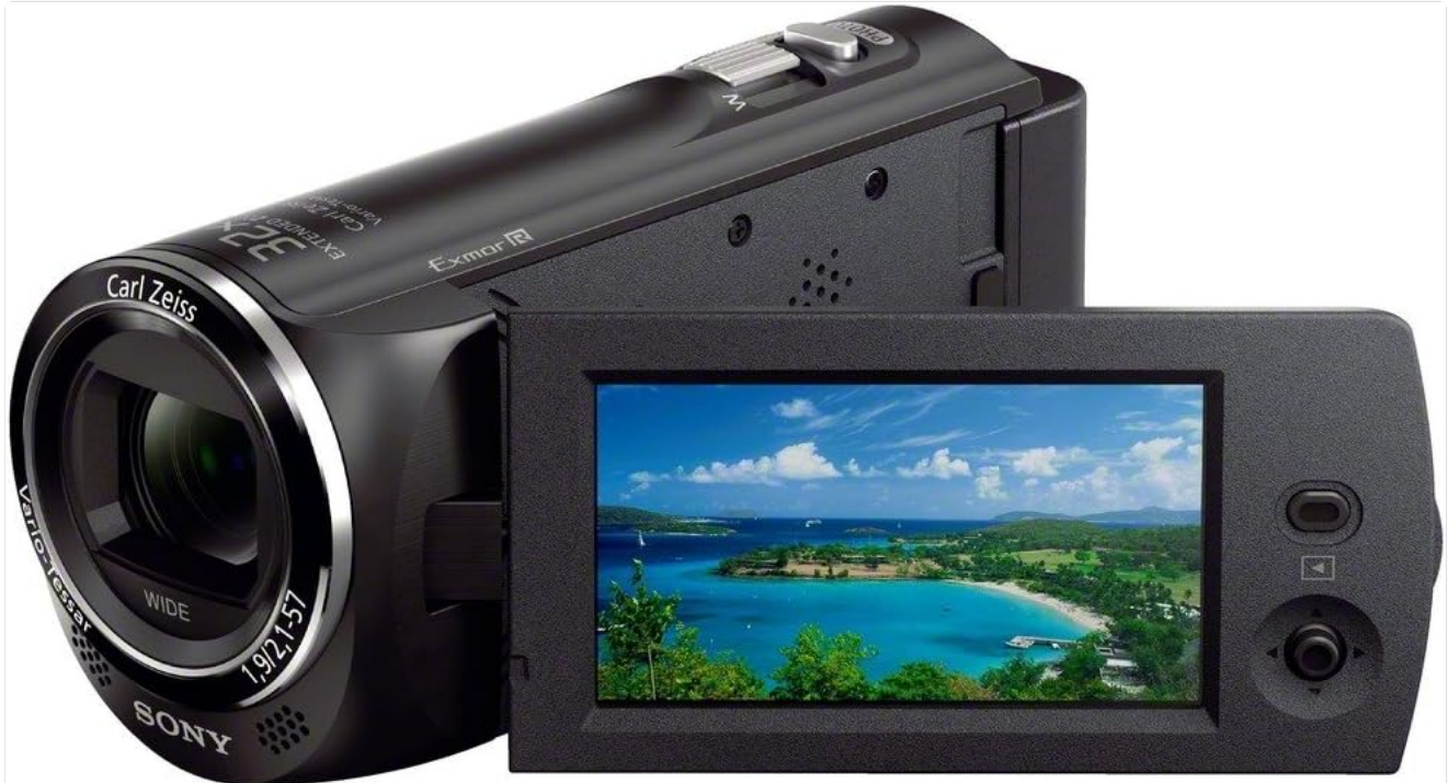
Figure 4.1: View of the Sony HDR-CX230 Handycam with its LCD screen open, revealing the control buttons and joystick on the screen bezel. This interface is used for menu navigation and playback.
