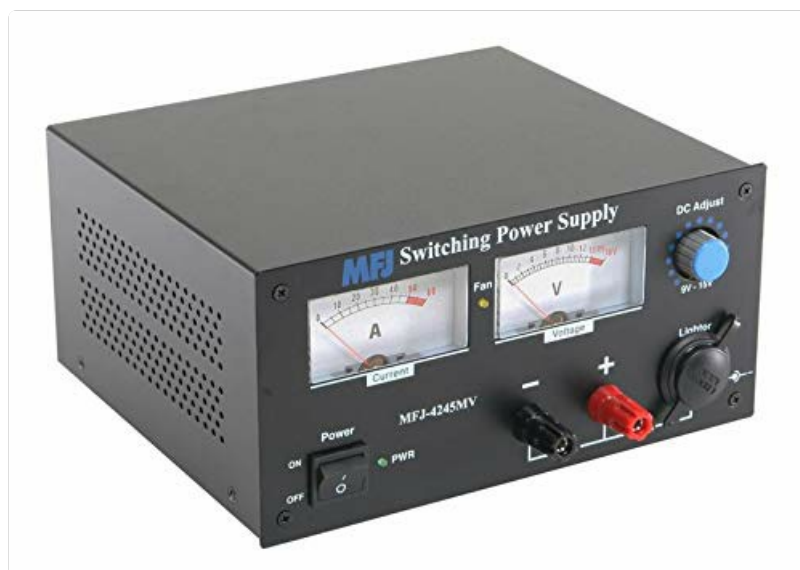
Figure 1: Front panel of the MFJ-4245MV power supply. This image displays the current (A) and voltage (V) meters, the power ON/OFF switch, the DC Adjust knob for voltage control (9V-15V), and the main 40A output terminals (red for positive, black for negative). A lower current 7A output terminal and a lighter socket are also visible.
