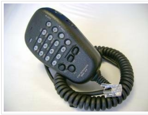
Image: The YAESU MH-48A6JA DTMF Hand Microphone. This image displays the black handheld microphone unit, featuring a numeric keypad with additional alphabet characters for APRS/Packet use, along with several function buttons. A coiled cord extends from the microphone, terminating in an RJ-style modular connector, which is used to connect the microphone to compatible Yaesu transceivers.
