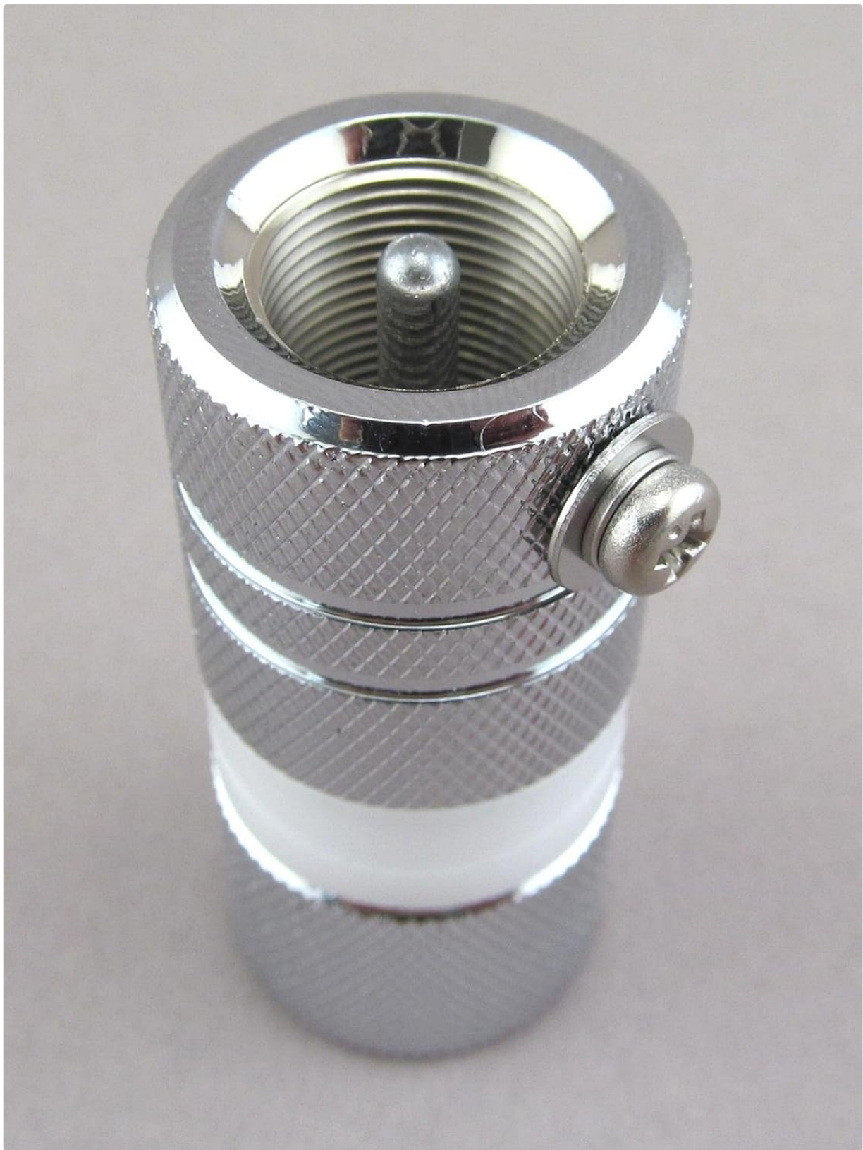
Figure 2: View of the Comet AD-35M adapter, highlighting the 3/8"-24 threaded stud for antenna attachment and the side-mounted grounding screw for electrical connection to a ground plane or chassis.
