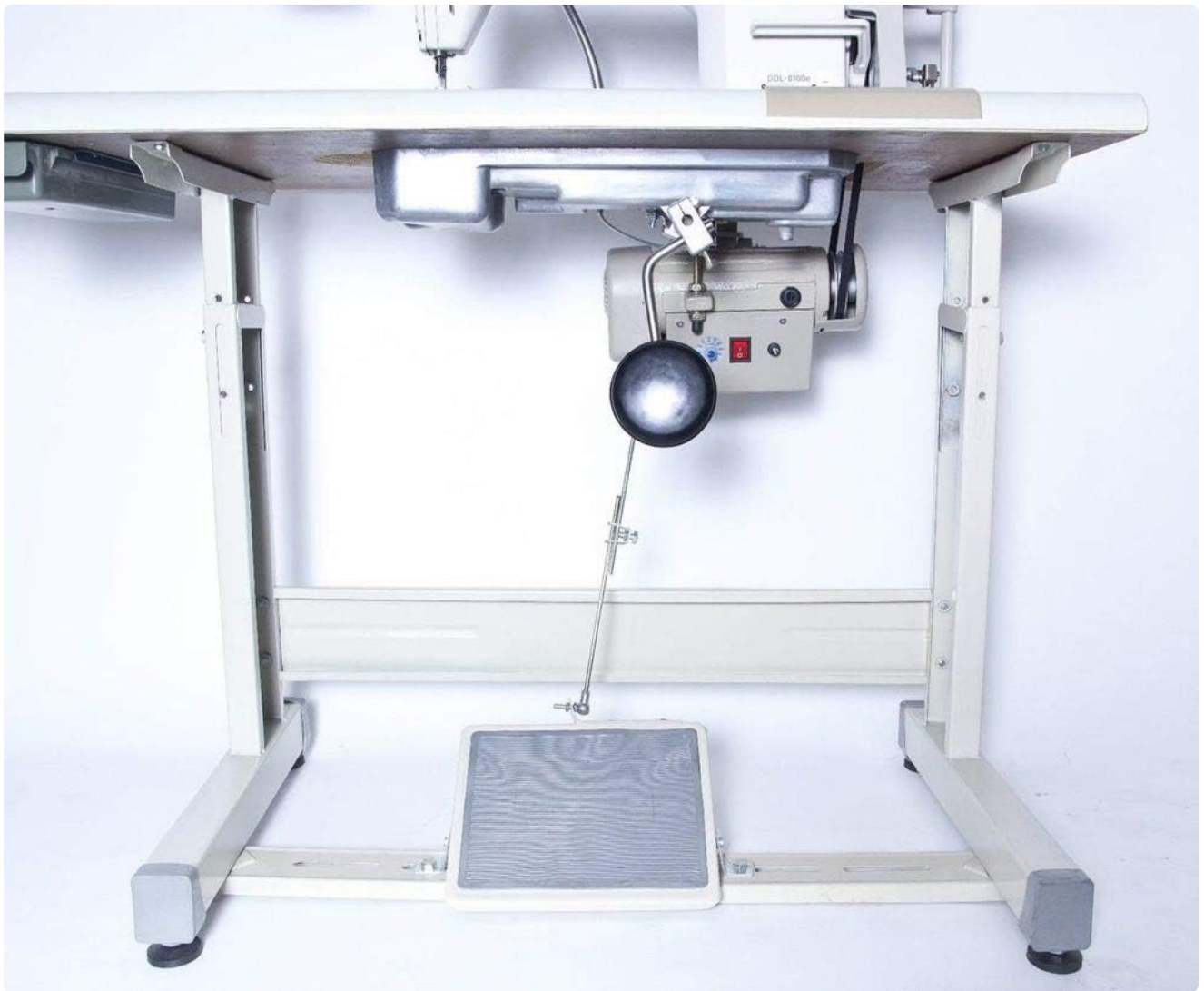
Figure 2.3: Underside view of the sewing machine table, showing the installed foot pedal and servo motor mechanism.
