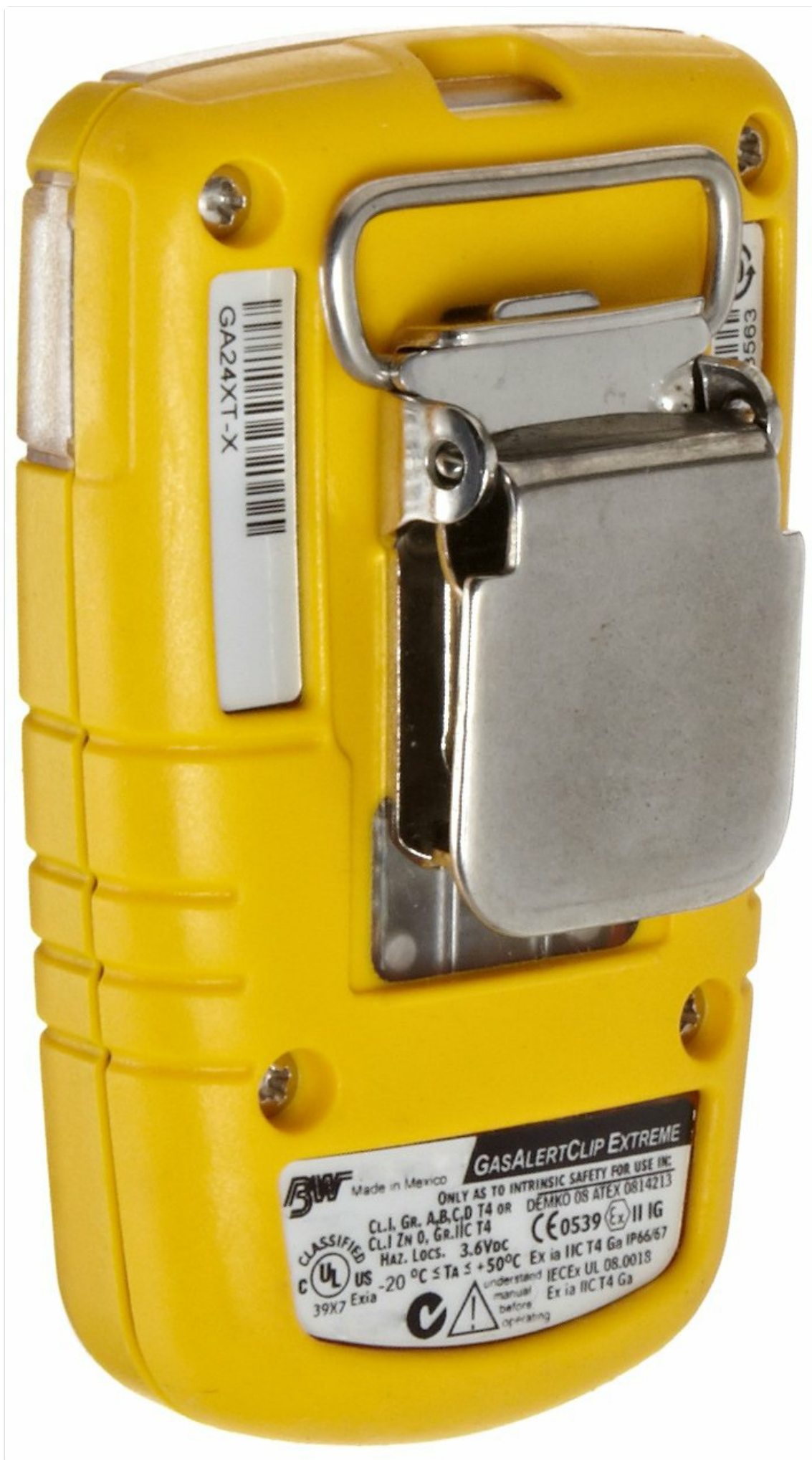
Figure 2: Back view of the GasAlertClip O2 detector, highlighting the robust metal alligator clip for secure attachment and regulatory
