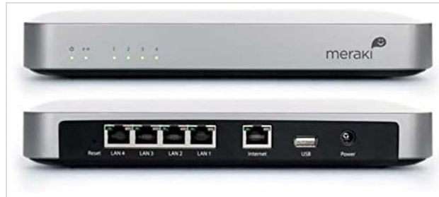
Figure 3.1: Front and rear view of the Cisco Meraki MX60, illustrating the power input, USB port, Internet (WAN) port, LAN ports (1-4), and reset button on the rear panel, along with front panel LEDs.
