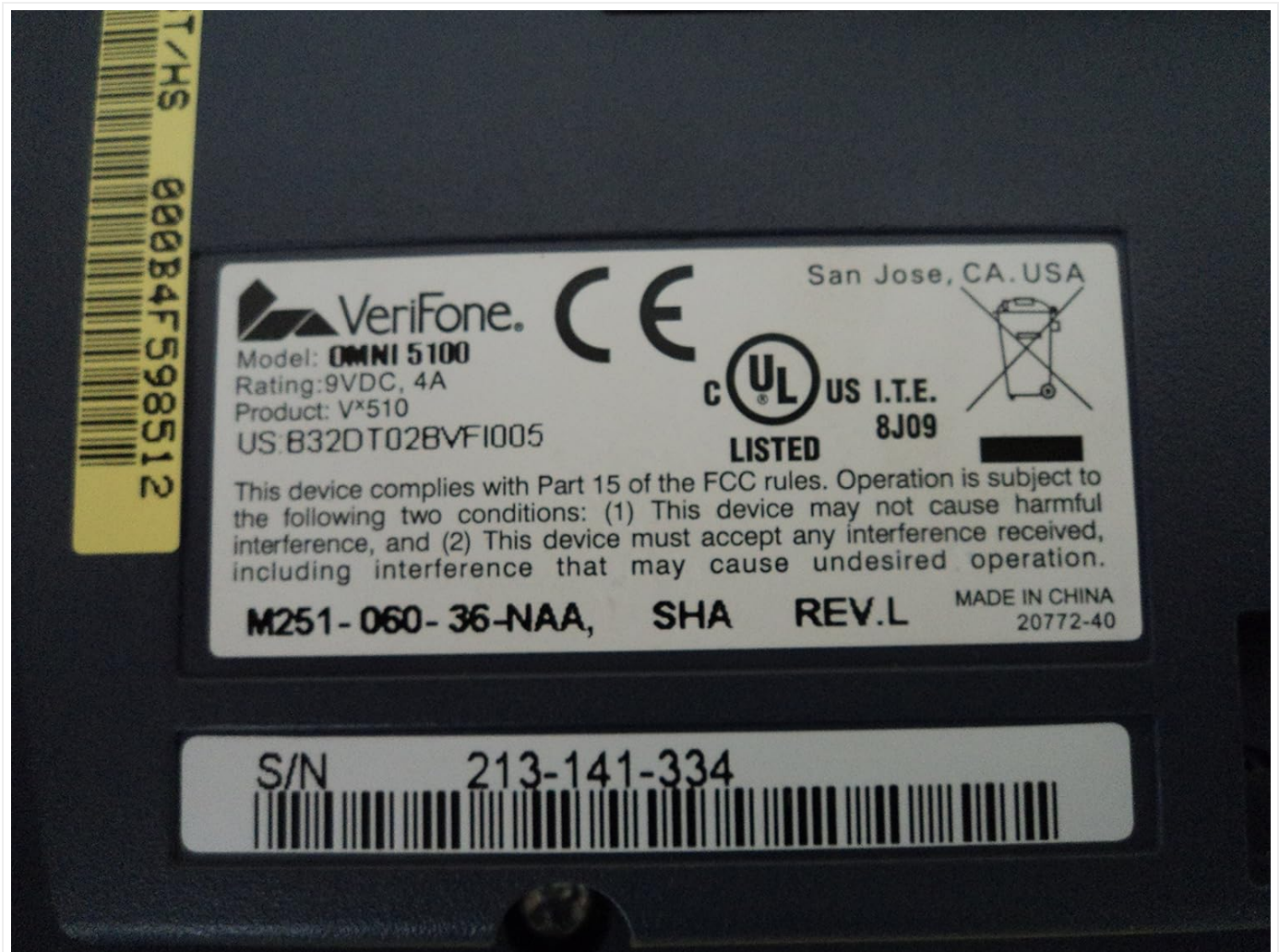
Figure 6: Bottom label of the VeriFone VX510 terminal, showing model number M251-060-36-NAA, product rating, and serial number (S/N 213-141-334).
