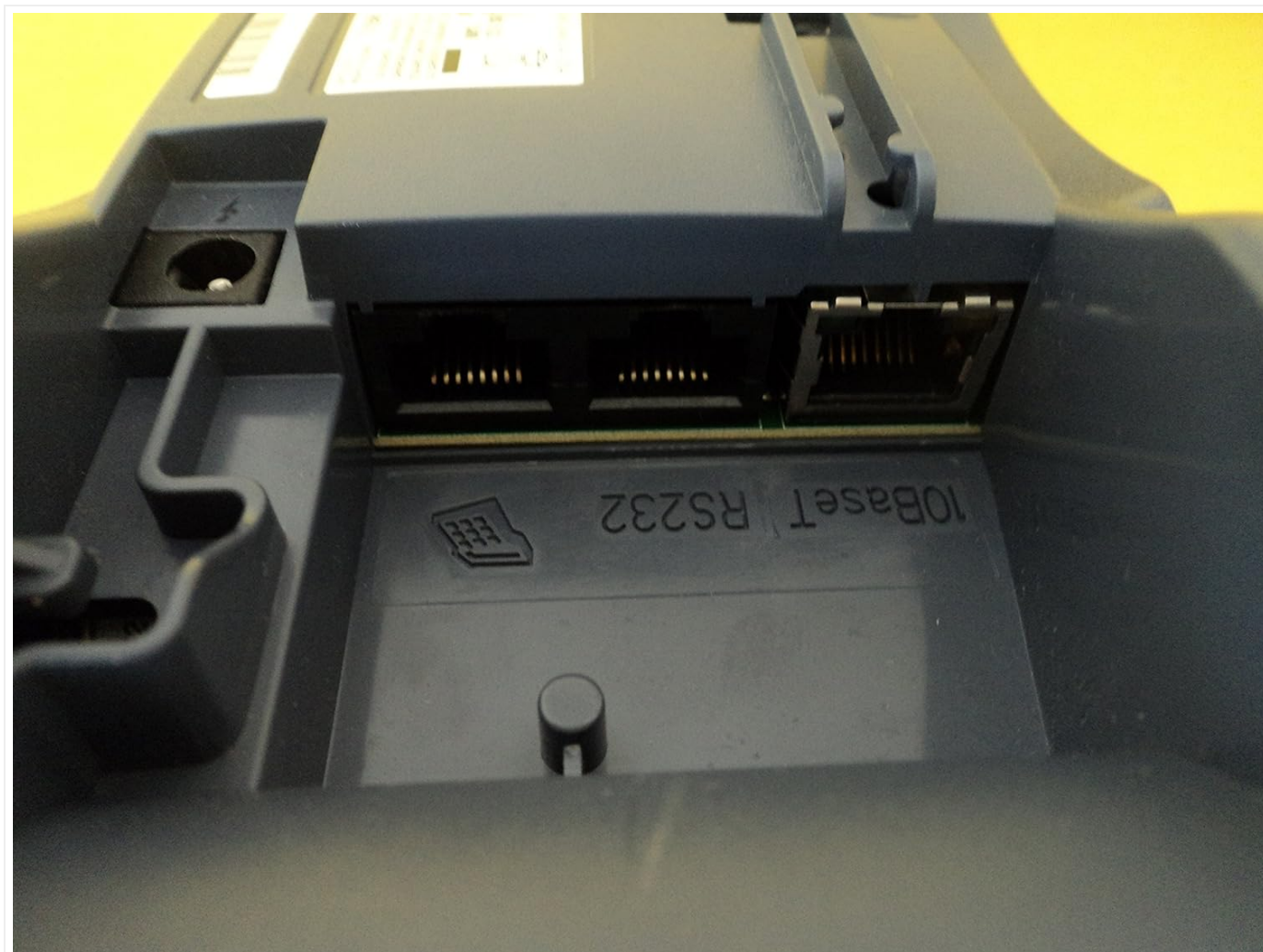
Figure 4: Rear view of the Verifone VX510, showing the communication ports, including 10BaseT (Ethernet) and RS232 connections.
