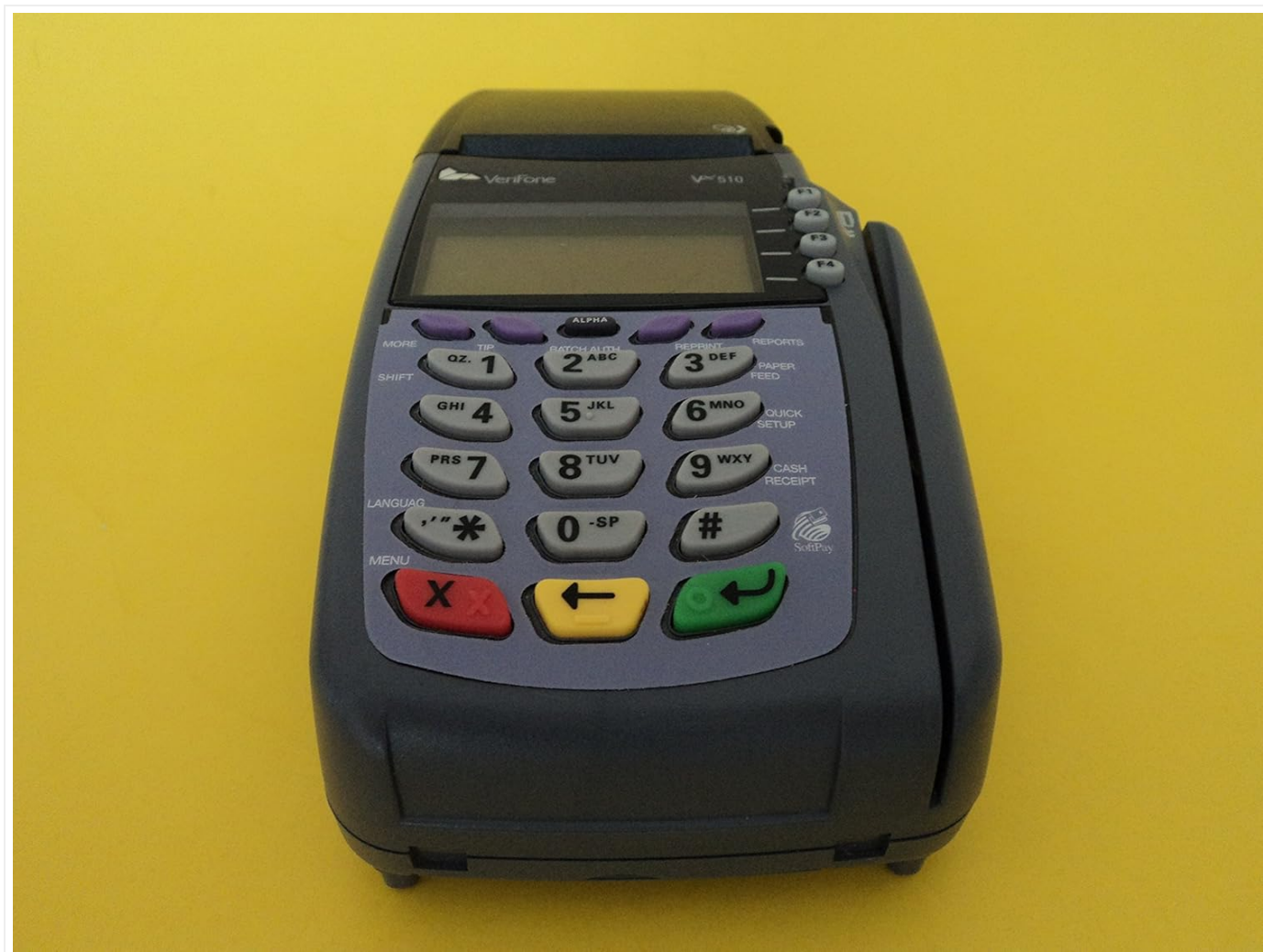
Figure 2: Front view of the Verifone VX510 terminal, highlighting the keypad and display screen.
