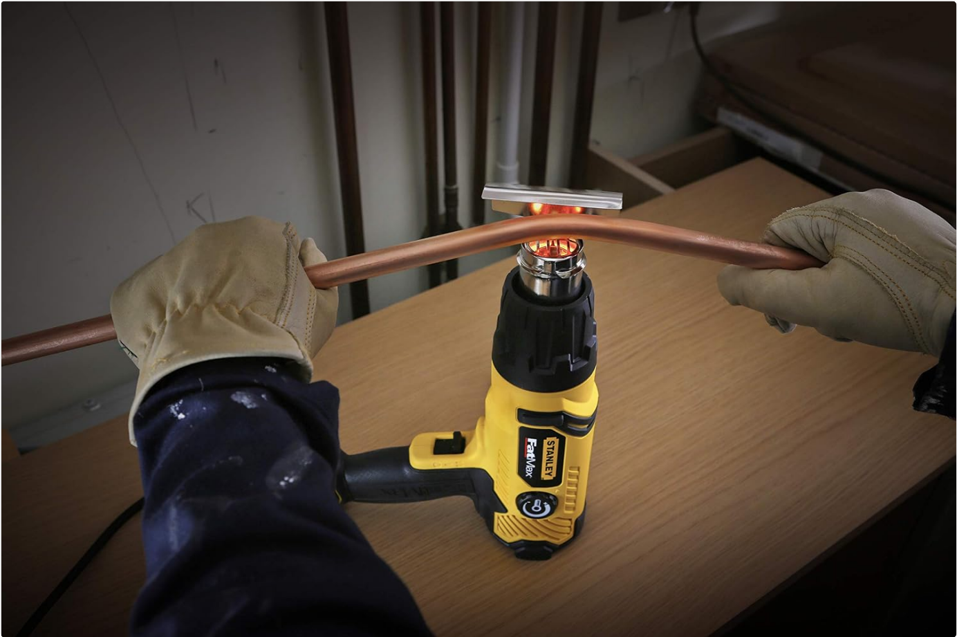
Figure 5.1: The hot air gun positioned for hands-free operation, demonstrating its use in heating and bending a copper pipe.
