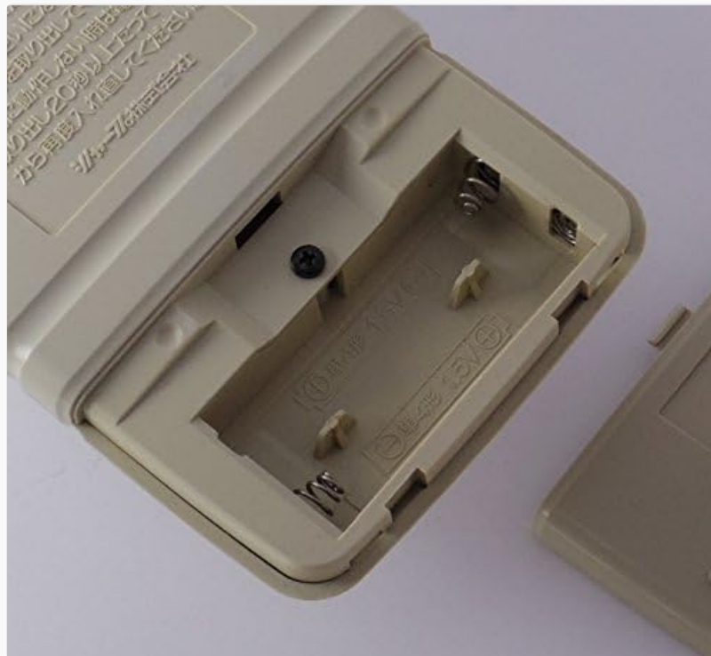
Image 4.1: The open battery compartment of the SHARP A419JB remote control, showing the slots for two AAA batteries and the polarity markings.
