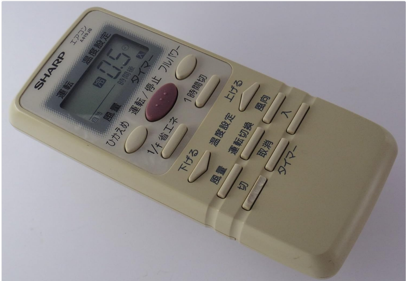
Image 3.1: Front view of the SHARP A419JB remote control, showing the LCD display and all control buttons. The display shows temperature settings and operational status. The central button is for power on/off, surrounded by various function buttons.
