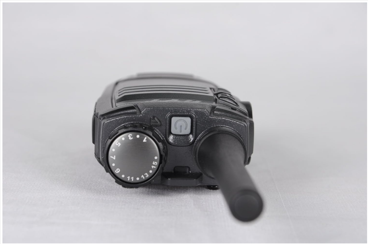
Image 3.3: Top view of the Hytera TC-320U-1 radio, showing the channel selector knob (numbered 1-16) and the power/volume knob.
