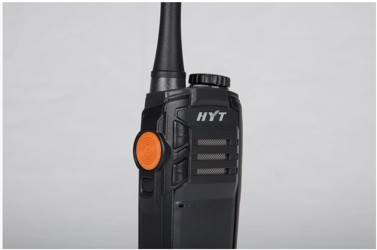
Image 3.2: Side view of the Hytera TC-320U-1 radio, highlighting the orange Push-To-Talk (PTT) button.
