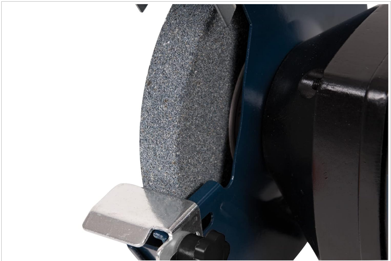
Figure 7: Close-up of the coarse P36 grinding wheel, typically used for aggressive material removal and initial sharpening.
