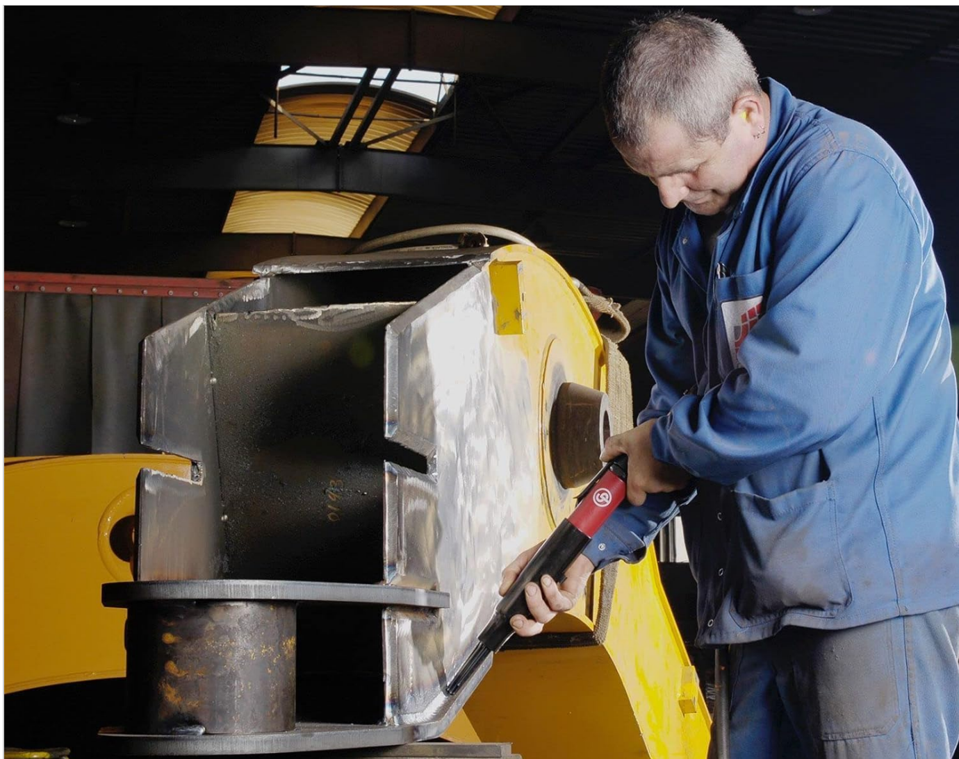
Figure 2: A worker demonstrating the use of the CP7115 Needle Scaler on a large metal structure. This illustrates the tool's application in industrial settings for surface preparation.
