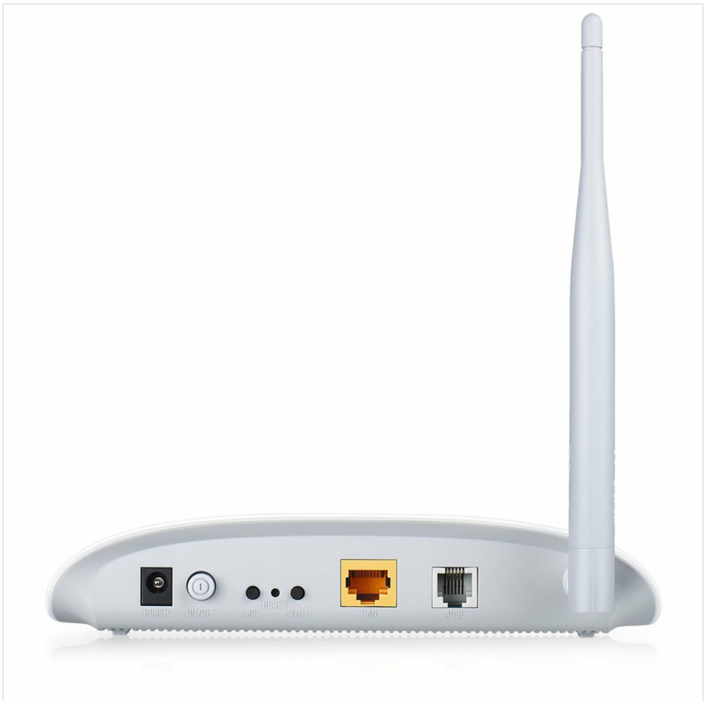
Figure 2: Rear view of the TD-W8151N showing ports and buttons.
