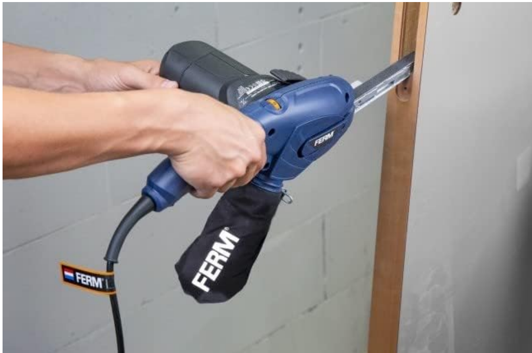
Figure 5.1: Demonstrates the FERM Precision Belt Sander in use, highlighting its ability to reach into narrow spaces, such as sanding a door frame.
