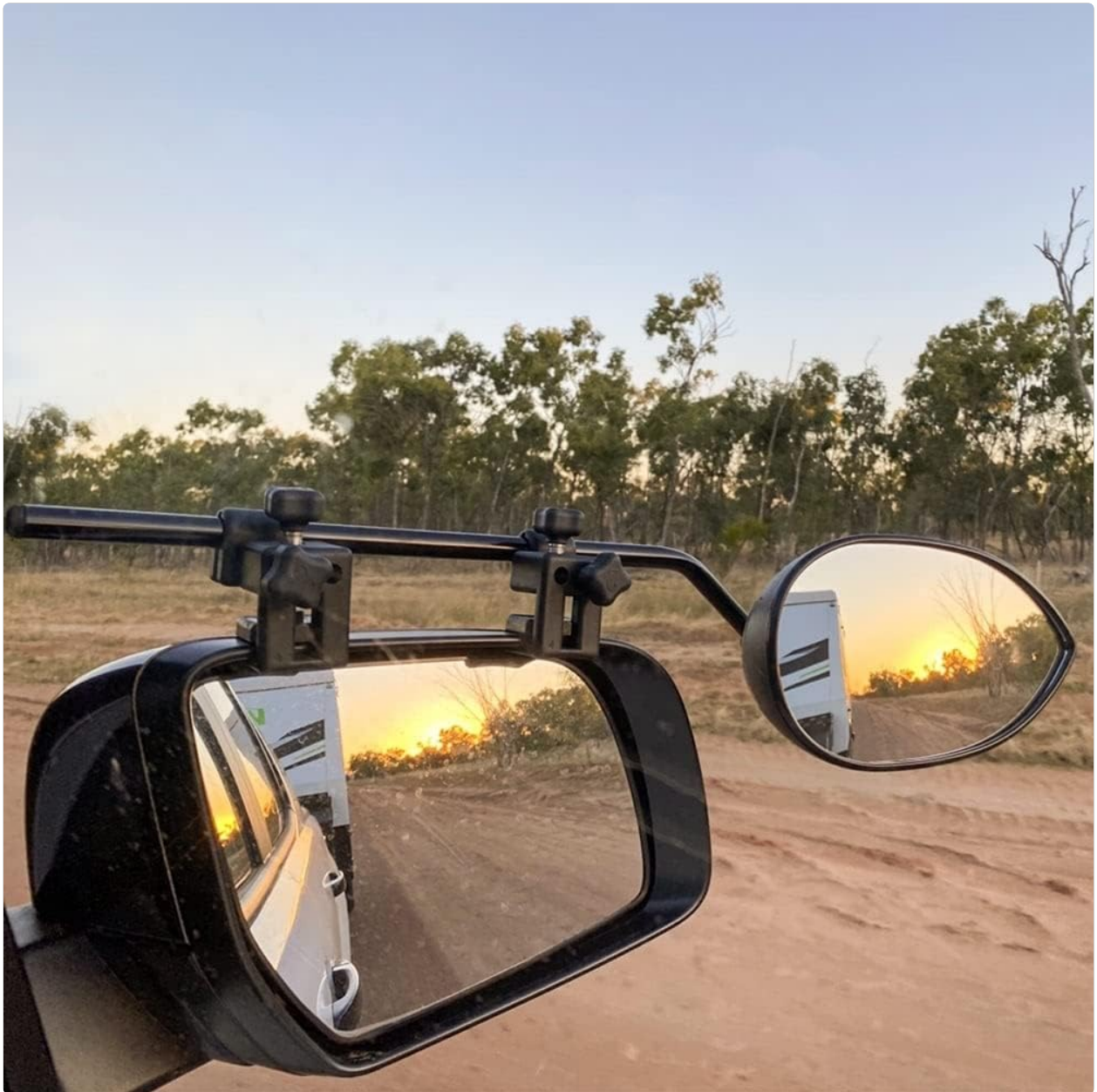
Image 3.2: A driver's view through the Milenco Aero 4 mirror, demonstrating visibility of a towed vehicle against a sunset backdrop.
