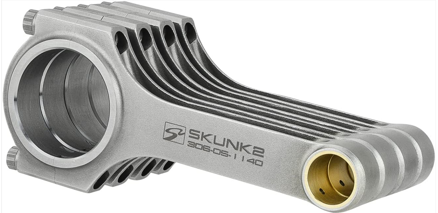
Figure 1: A single Skunk2 Racing Alpha Series Connecting Rod, showcasing its H-beam design and bronze wrist pin bushing.
