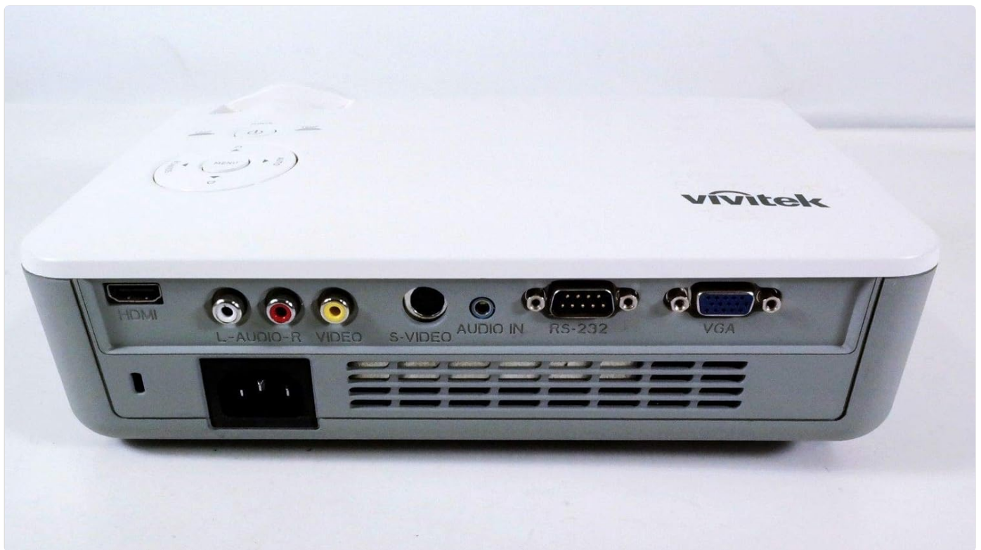
Figure 2.1: Rear view of the Vivitek D519 Projector, highlighting the HDMI, VGA, S-Video, and audio input ports.
