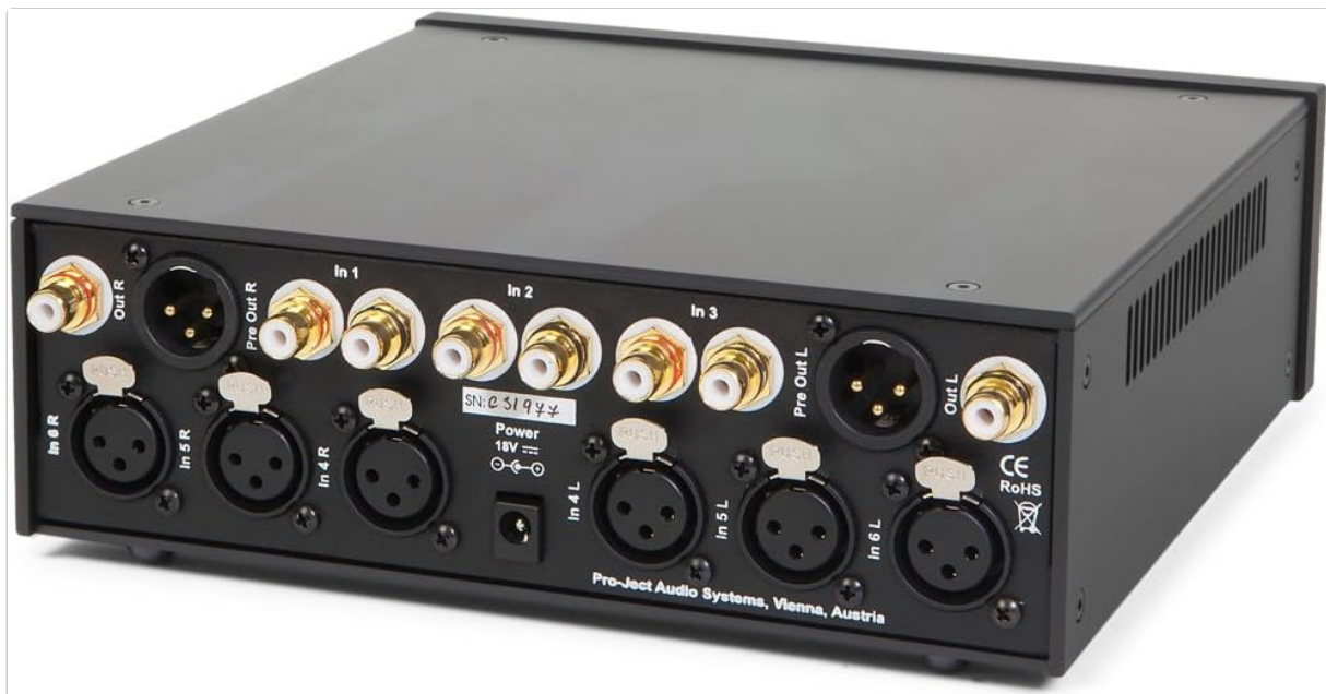
Image 1: Rear Panel Connections. This image displays the rear panel of the Pro-Ject Pre Box RS preamplifier. Visible connections include RCA inputs (In 1, In 2, In 3), XLR inputs (In 4 L/R, In 5 L/R, In 6 L/R), RCA outputs (Out R, Pre Out R, Out L, Pre Out L), and the 18V power input. The serial number and manufacturer information are also visible.
