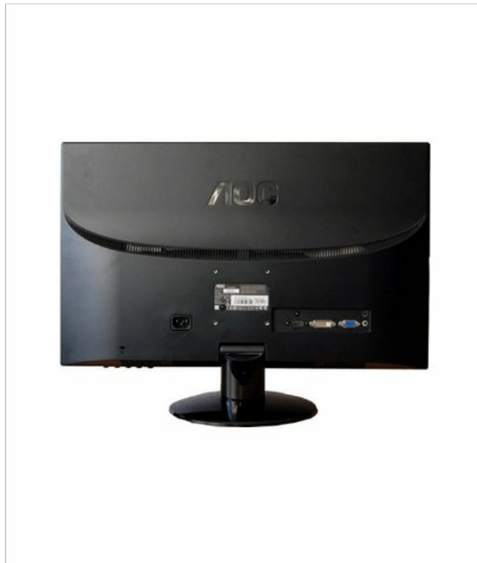
Figure 2.3.2: Rear view of the AOC e2352Phz monitor. This image highlights the various input and output ports located on the back panel, including power, video (VGA, DVI, HDMI), and audio connections.
