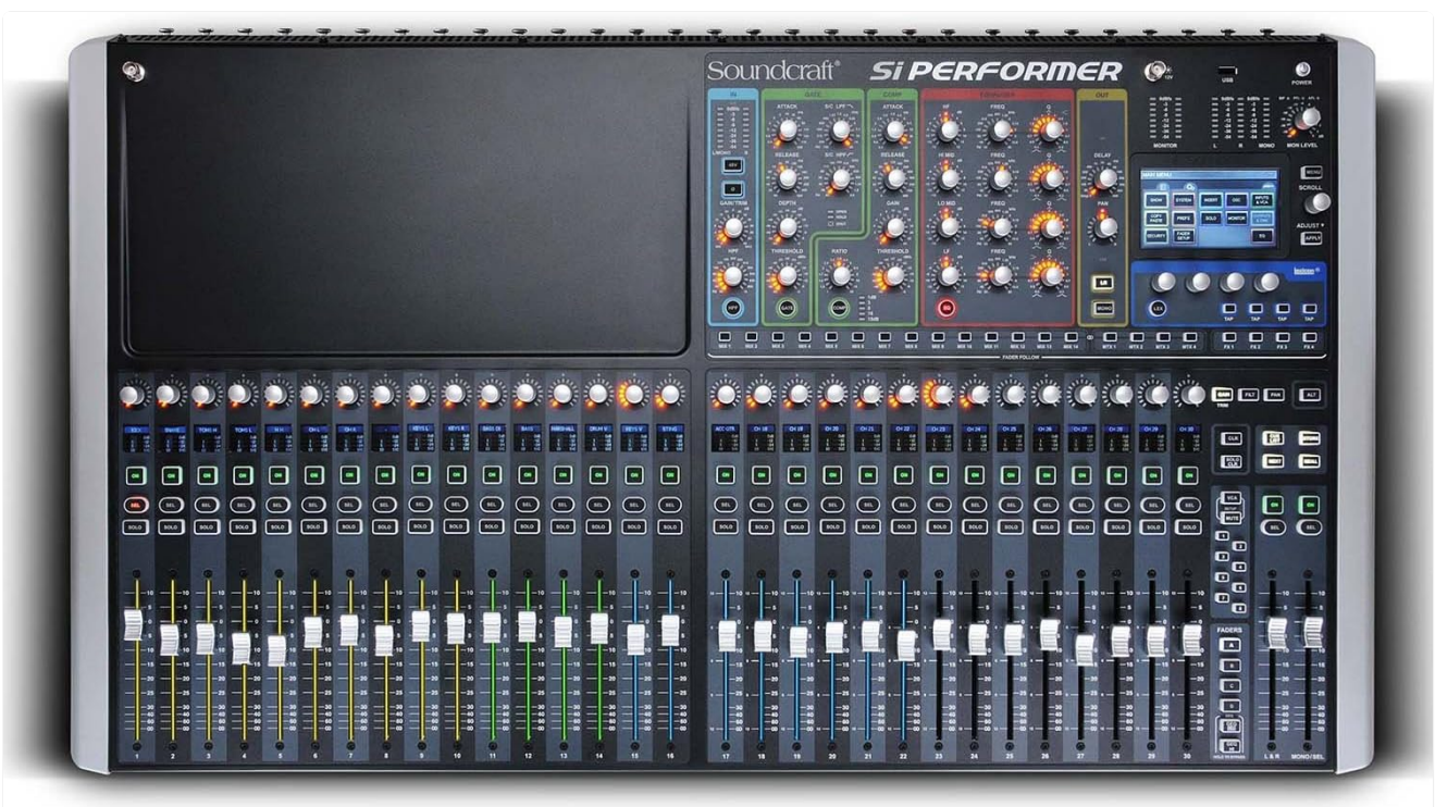
Figure 1: Front view of the Soundcraft Si Performer 3 Digital Mixer, showcasing the faders, control knobs, and display screens.
