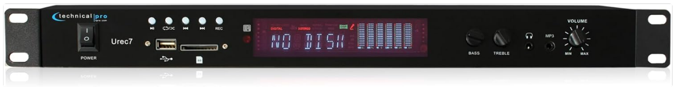
Figure 3.1: Front Panel of the UREC7. This image displays the front of the Technical Pro UREC7, showing the power switch, USB and SD card slots, control buttons (play, pause, stop, next, previous, record), LED display, bass and treble knobs, headphone jack, and master volume control.
