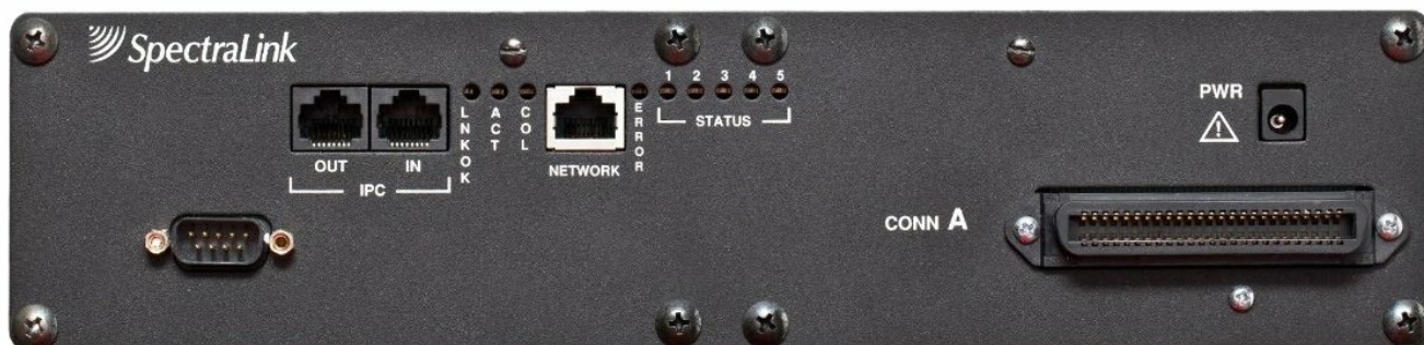
Image showing the Spectralink 8000 Telephony Gateway TGD208 unit, highlighting its compact design and port layout.
