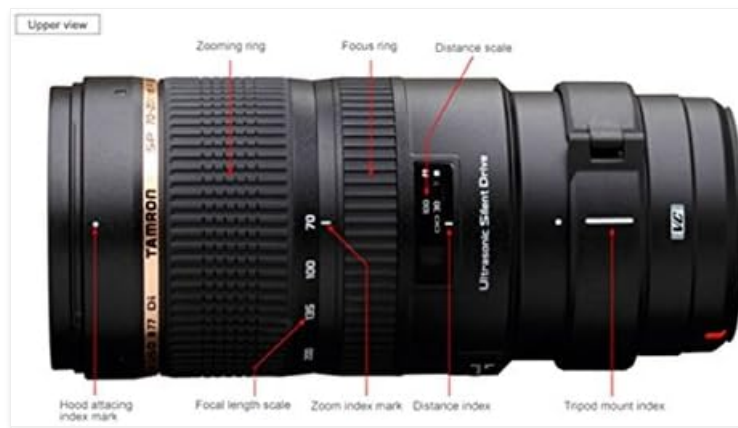
Figure 2: Upper view of the lens with labeled components.
