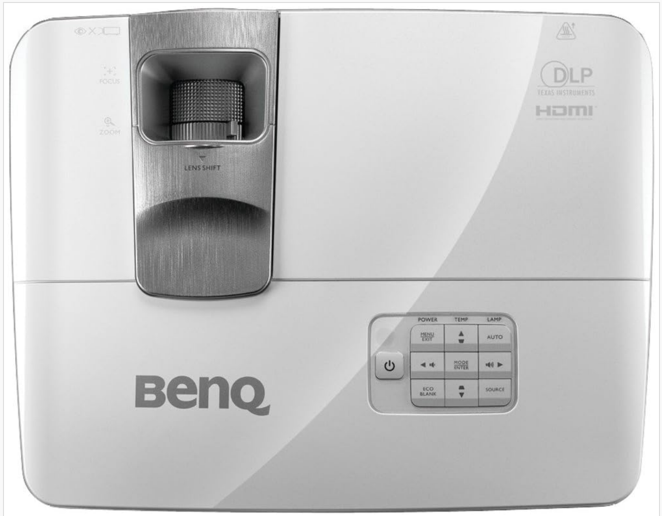
Figure 3.2: BenQ W1070 Projector (Top View with Lens Shift Mechanism)
