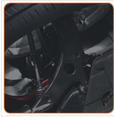
Image: A view of a vehicle's suspension, showing the location of a control arm.
