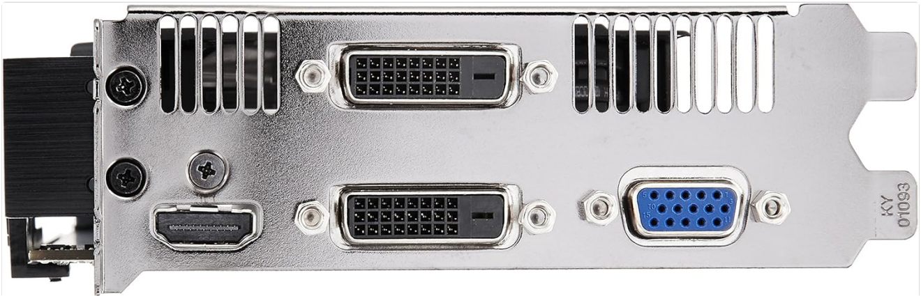
Figure 2: Rear view of the ASUS GTX650TI-O-1GD5 Graphics Card, highlighting the various display output ports including DVI, HDMI, and VGA. This image helps identify the available connectivity options for monitors.
