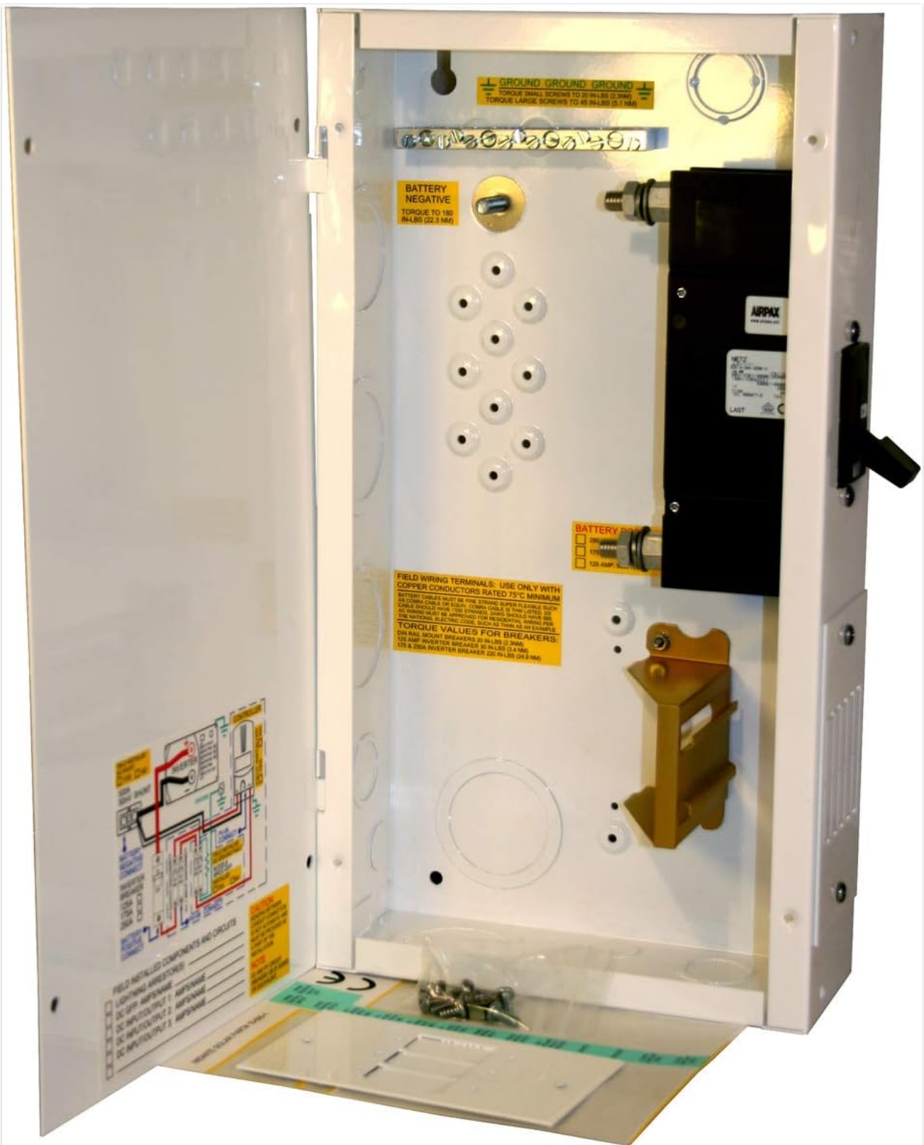
Figure 3.2: An internal view of the MidNite Solar MNDC250 Mini-DC Disconnect, highlighting the 250A/125VDC breaker, DIN rail slots, ground bus bar, and various connection points. The white powder-coated aluminum chassis is visible, along with labels for battery negative and ground connections.
