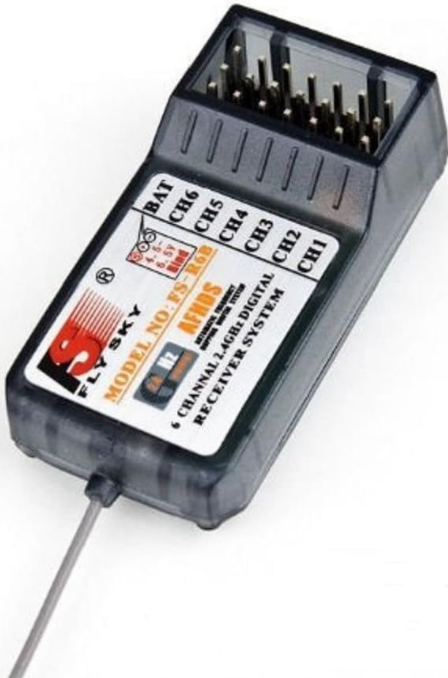
Figure 1: Top view of the FS-R6B receiver, illustrating the channel ports (CH1-CH6) and the BAT/BIND port. The antenna wire extends from the side.
